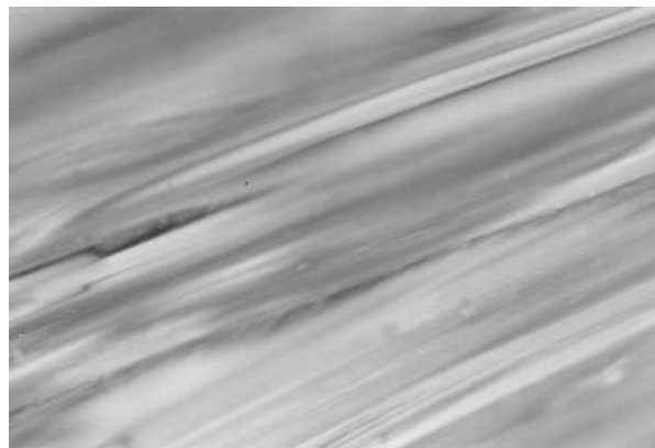
Figure 8. Photomicrograph of several strands of hand-drawn fiber of copolymer I-1 displaying a highly oriented fibrillar morphology (magnification 400 \times ; reproduced at 70% of original size).
